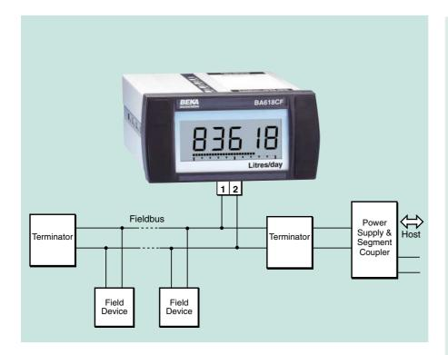
The BA618CF-F Fieldbus Indicator is a new cost-effective panel mounting instrument that displays a single fieldbus variable in a control room or process area. Housed in a robust panel mounting enclosure with an IP66 front, the instrument has a large, high contrast five digit display and a horizontal bargraph. The BA618CF-F indicator uses the same technology and compliments the well established BEKA eight variable fieldbus displays that are now in worldwide use.
